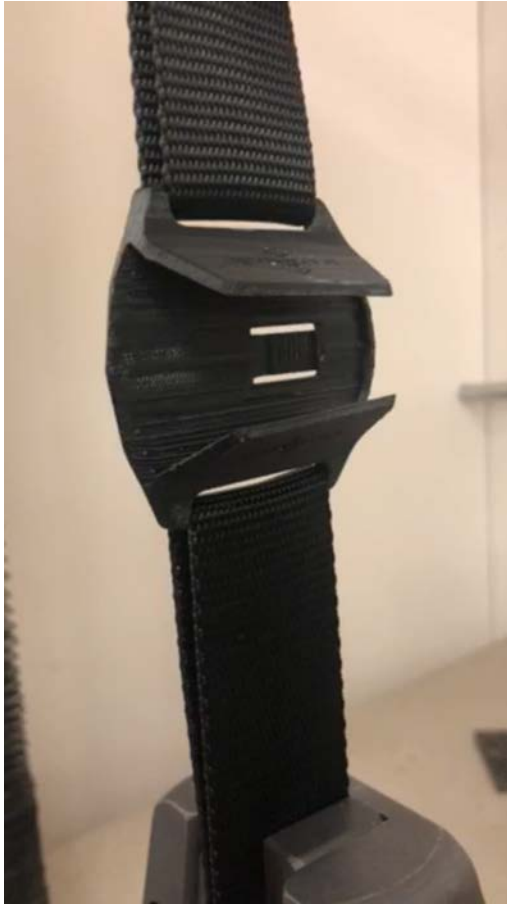
Holster with nylon webbing securing it into the jaws of the testing machine.
